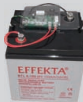
Battery line on rail prepared for integration into a Quasar
