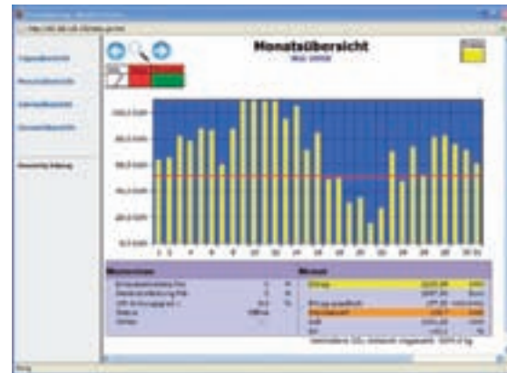
Graphical and tabulation view of daily, monthly and total values, reference value for annual yield, input voltage in daily view available. (German language screenshot).
