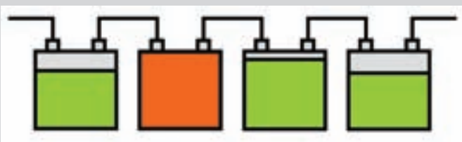
Fig. 2: Standard charging of the batteries using traditional methods causes overcharging or deep discharging and damage to individual batteries, which in turn compromises the reliability of the entire system.
