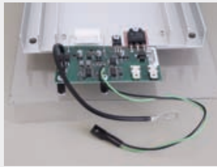
detail: board with temperature sensor
