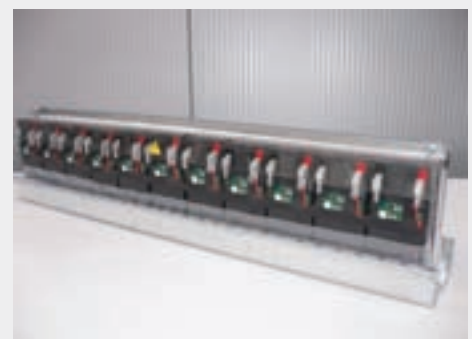
Battery line on rail prepared for integration into a Quasar
